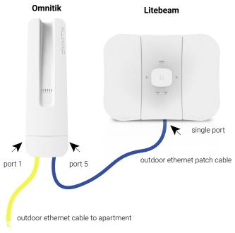
That brings us to another important aspect of OmniTiks: they can be used to connect to other devices. The image to the right shows the five ethernet ports on an OmniTik. The port farthest to the left carries power and data from your apartment to the OmniTik. The other ports can either be used to connect to another Mesh-connected device, usually a LiteBeam, or to connect to other apartments in your building, so let your neighbors know that they can join NYC Mesh today!
