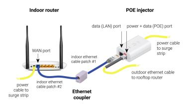
If the PoE injector is on (indicated with a green light) and there is still no power at the LiteBeam, check that the ethernet cable leading to the rooftop antenna is properly plugged into the PoE injector (try unplugging and plugging back in, it should click into place).
